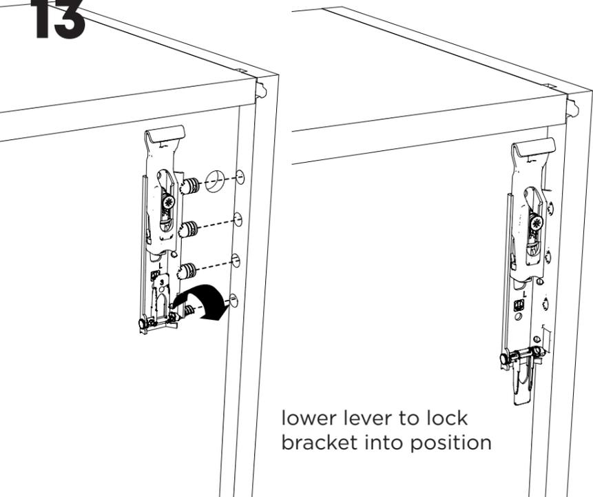
lower lever to lock bracket into position
