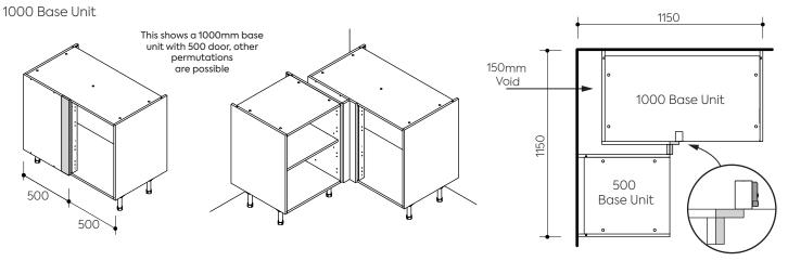
Both parts of the corner post are fitted together using chipboard screws (not supplied) to form an 80 x 80mm right angled assembly.
