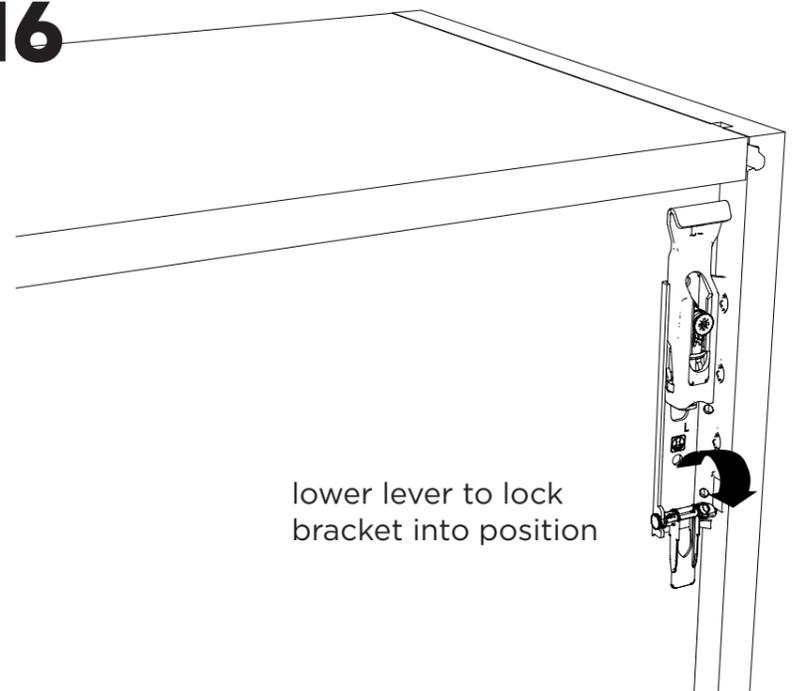
lower lever to lock bracket into position
