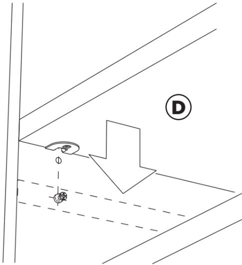
**8** Using a screwdriver tighten Connector Housings.
