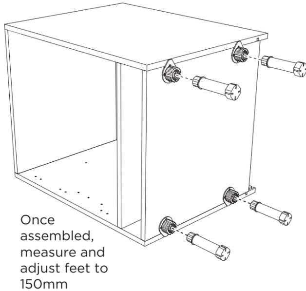
Once assembled, measure and adjust feet to 150mm
