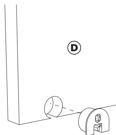
**7** Insert Rafix Bolts into both End Panels, then install Fixed Shelf D.
